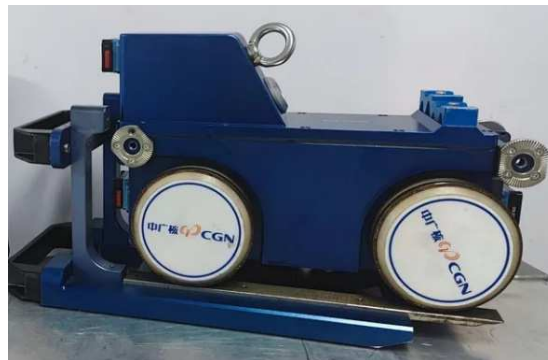
Figure 4. Inspection robot hardware implementation.
